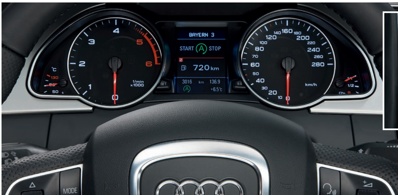
The start-stop status is shown in the dash display, left, and can be disabled at the push of a switch, above
